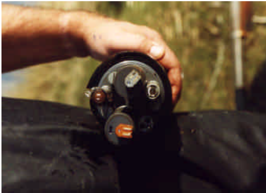
Figure 2. Wiped sensor tips at end of a three week deployment. Note the rings of biological fouling at the wiped periphery: demonstrates the value of YSI wiped technology.
