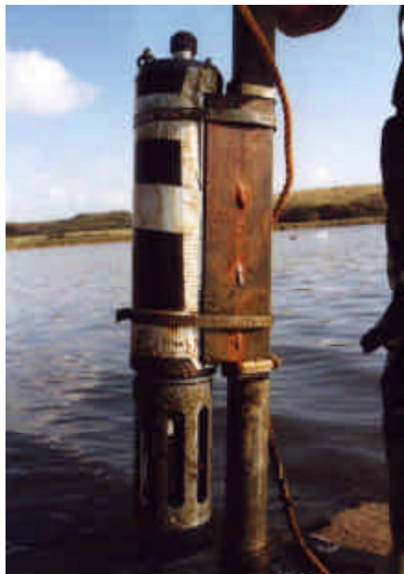
Figure 1. The YSI 6600 instrument affixed to the deployment apparatus after a three week deployment.
