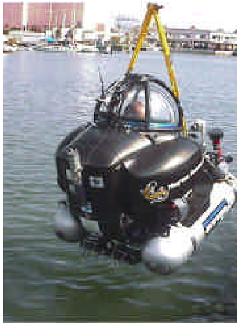
A YSI 6600 multiparameter sonde is shown attached to the front of the SSE Deep Worker 2000 submersible vehicle.
